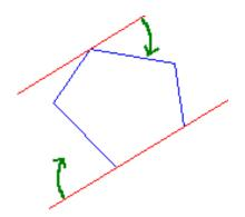
Then the two straight edges are rotating till one hits again the polygon.
