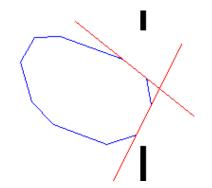
Before the polygon goes through the door, the tangents are crossing on the right side of the polygon.
